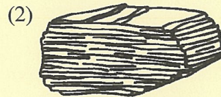
Easily split layers of 0.0001-cm-diameter particles cemented together
