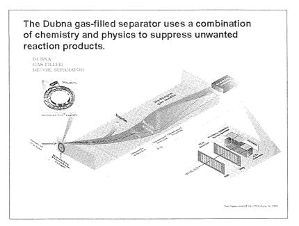
Strong magnetic fields in the separator can focus the elements being searched for and separate them from the large number of intervening reaction products also created.
