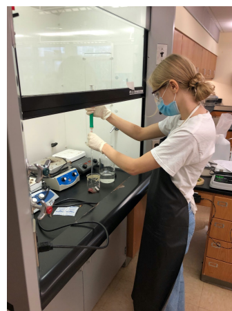
Fig. 5. Wet peroxide oxidation taking place within the fume hood
